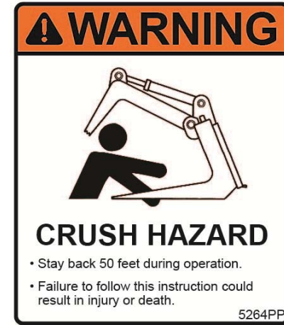
5264PP – CRUSH HAZARD WARNING LABEL
